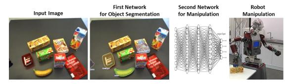
Figure 1 The input image is processed by the first deep network to segment and detect objects. The second network will output how and where to push one of the detected objects by the robot.
