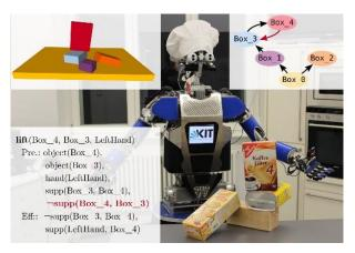
The humanoid robot ARMAR-III extracts objects and physically plausible support relations between them from its depth camera. These relations are needed for planning and prediction.
