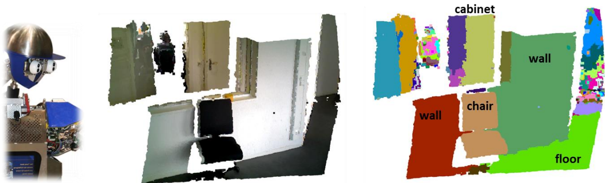
Figure 1: Deep learning for semantic scene and action perception. On the left the humanoid robot ARMAR-IIIa observes a scene including a chair, walls and cabinets. The aim here is to extract and label individual scene segments. For instance, the brown segment (see image on the right) represents the chair shown in the middle.
