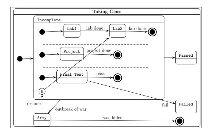
When re-entering composite state, establishes the last active configuration
