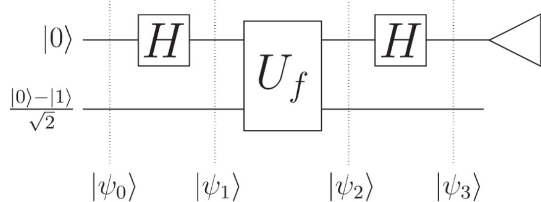
$$|\phi_1\rangle = \left( \frac{1}{\sqrt{2}}|0\rangle + \frac{1}{\sqrt{2}}|1\rangle \right) \left( \frac{|0\rangle - |1\rangle}{\sqrt{2}} \right) = \\ \frac{1}{\sqrt{2}}|0\rangle \left( \frac{|0\rangle - |1\rangle}{\sqrt{2}} \right) + \frac{1}{\sqrt{2}}|1\rangle \left( \frac{|0\rangle - |1\rangle}{\sqrt{2}} \right)$$
